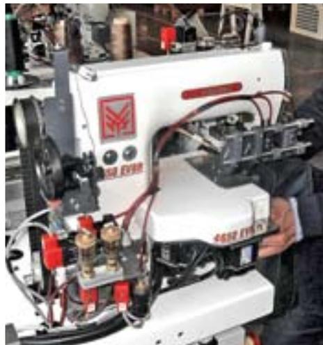
An earlier version of the 4650EV9R belt loop setter, now comes equipped with a 7 inch touch screen panel
